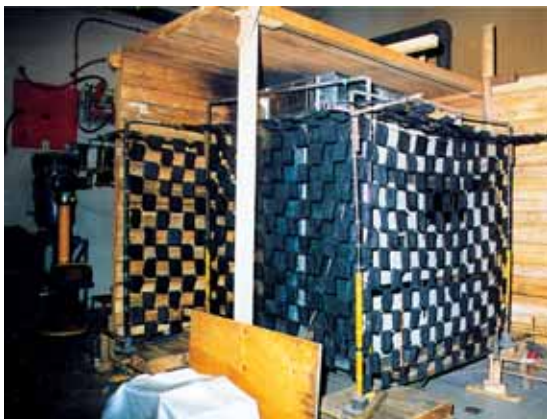
Preparation of the fabric indicators for the arc proof test.
